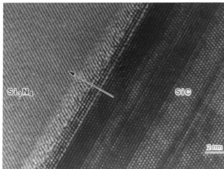
Fig. 6. HREM image (200 kV) of the same interfacial boundary displayed in Fig. 5, taken approximately 20 nm away from the region shown in Fig. 5. The image reveals direct bonding between the whisker and the \beta\text{-Si}_3\text{N}_4 matrix grain with no indication of amorphous phase present. Orientation of constituents corresponds to Fig. 5. The scan path of the focused probe (see Fig. 8) is indicated by the arrow. From Ref. 36.
